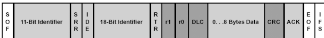
Figure 3. Extended CAN: 29-Bit Identifier
