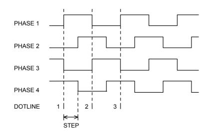
There are four different positions for the stepper motor. The driving is bipolar and can be achieved with circuits like Rohm BA6845FS. Please refer to the IC's data sheet for further informations. It is recommanded not to exceed 0.2v like voltage drop in the stepper motor driver circuit.
